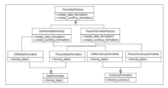
Comparing that image to the simpler text above it shows that a picture is not always worth a thousand words, after all, especially considering we haven't even allowed for factory selection code here. Of course, in Python, we don't have to implement any interface classes, so we can discard DateFormatter, CurrencyFormatter, and FormatterFactory. The formatting classes themselves are pretty simple:
