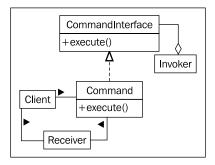
A common example of command pattern in action is actions on a graphical window. Often, an action can be invoked by a menu item on the menu bar, a keyboard shortcut, a toolbar icon, or a context menu. These are all examples of Invoker objects. The actions that actually occur, such as Exit, Save, or Copy are all command implementations of CommandInterface. A GUI Window to receive exit, document to receive save, and ClipboardManager to receive copy commands are all examples of possible Receivers.
