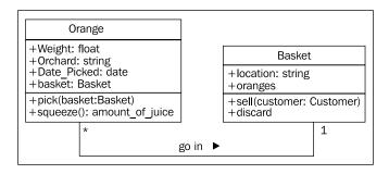
Adding models and methods to individual objects allows us to create a **system** of interacting objects. Each object in the system is a member of a certain class. These classes specify what types of data the object can hold and what methods can be invoked on it. The data in each object can be in a different state from other objects of the same class, and each object may react to method calls differently because of the differences in state.
